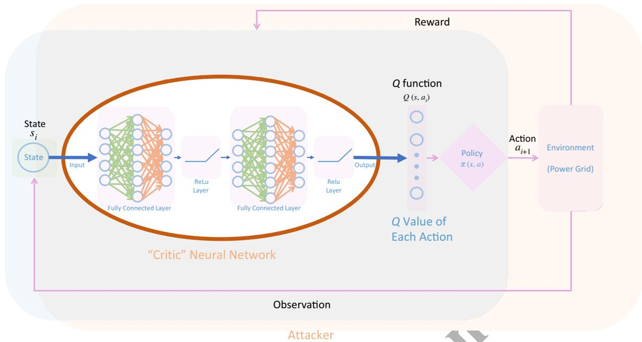
F10:1 FIG. 10. Structure of deep  $Q$ -learning algorithm used in this paper. Structure describes the processes inside the attacker block in Fig.
